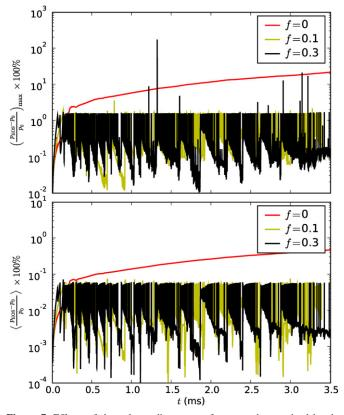
**Figure 7.** Effects of the volume discrepancy factor as characterized by the percent difference between the thermodynamic pressure as given by the equation of state,  $p_{\text{EOS}}$ , and the base state pressure,  $p_0$ , for the hot model. The top panel shows the maximum value whereas the bottom panel shows the average value of the percent difference in the computational domain. Note the different vertical scales between the two plots.
