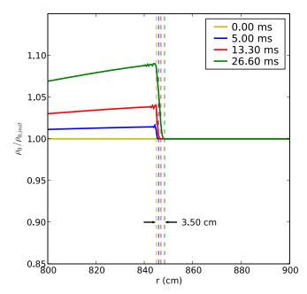
**Figure 6.** Expansion of the base state due to heating. Plotted is the ratio of base state density,  $\rho_0$ , to the initial (t = 0) base state density,  $\rho_{0,\text{init}}$ , near the surface of the atmosphere for the cold model. We define the surface to be where  $\rho = \rho_{\text{cutoff}}$  and it is represented by the vertical dashed lines. The base state has expanded 3.5 cm in 26.6 ms of evolution.
