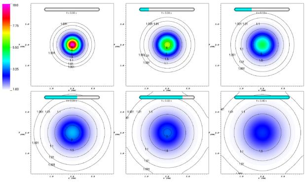
Figure 17. Time evolution of the diffusion of a two-dimensional Gaussian pulse of enthalpy as described in the text. The value of time displayed is the evolution time, *t*. This simulation was run with a  $1024 \times 1024$  grid with time step size  $\Delta t = 0.001$  s. Excepting edge effects near the domain boundary, the numerical solution maintains its axisymmetric form about the center of the pulse at (x, y) = (2.0, 2.0). (A color version of this figure is available in the online journal.)
