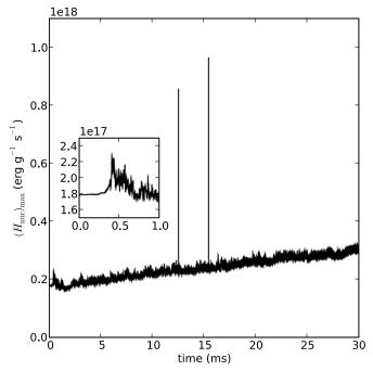
**Figure 15.** Plot of the maximum  $H_{\text{nuc}}$  in the cold model simulation as a function of time. The inset plot shows the early adjustment phase associated with Figures 9(b) and (c). The spikes are similar to that seen in the bottom panel of Figure 8, and are caused by the rapid burning of fresh fuel as it is brought into the burning layer by the turbulent convection.
