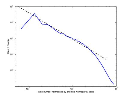
Fig. 2.— Kinetic energy wavenumber spectrum from a homogeneous isotropic turbulence simulation at 256<sup>3</sup>, taken from Aspden et al. (2008). The same forcing term used to maintain the turbulence is used in the present flame calculations. This figure demonstrates the range of scales captured by the ILES method for turbulent flow simulations at the resolution used in the present study. The dashed black line denotes the minus five-thirds decay expected in an inertial range.
