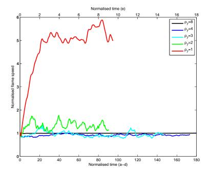
Fig. 7.— Normalized turbulent flame speeds. The time scale has been normalized by the laminar burning time, i.e. the time taken to burn one laminar flame width, specifically  $l_L/s_L$ . Cases (a)-(d) use the lower time scale; case (e), which has a significantly different evolution, uses the upper time scale. The turbulent flame speed has been normalized by the laminar flame speed.
