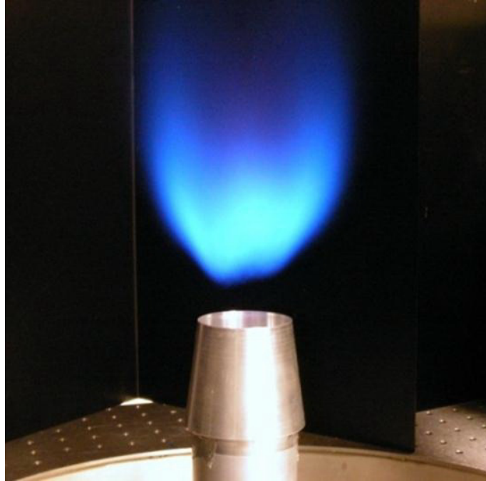
Figure 1. Lifted flame of the low-swirl burner.
