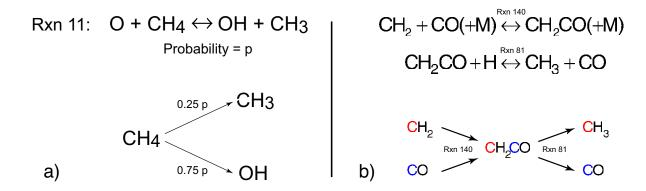
Figure 17: Examples of reactions involving molecules with several of the atoms being tracked. Example a) shows a symmetric case involving H atoms in CH<sub>4</sub>. Example b) show an unsymmetrical case involving carbon.
