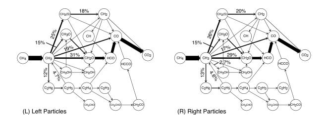
Figure 6: Carbon reaction path diagrams for vortex flame interaction,  $\phi = 0.8$ . Here only paths of strength > 1% of the largest path,  $CH_4 \rightarrow CH_3$ , are shown. For some paths of interest their weights are shown as a percent of the strongest.
