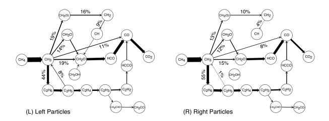
Figure 7: Carbon reaction path diagrams for vortex flame interaction,  $\phi = 1.2$ . Here only paths of strength > 5% of the largest path,  $CH_4 \rightarrow CH_3$ , are shown. For some paths of interest their weights are shown as a percent of the strongest.
