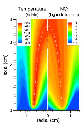
Figure 10: Temperature and NO mole fraction for the laminar nonpremixed flame. The dotted white line is the stoichiometric boundary between the fuel and air.
