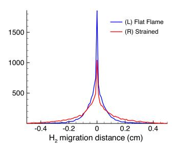
Figure 9: Symmeterized distributions of horizontal H<sub>2</sub> migration show how the flowfield strain disrupts local hydrogen chemistry in the rich flame.
