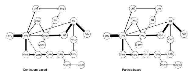
Figure 3: Reaction path diagrams for rich ( $\phi = 1.2$ ) premixed methane flame computed using PREMIX with GRI-Mech 3.0: continuum-based CHEMKIN rate evaluation, and particle-based tabulation of 80,000 trajectories.
