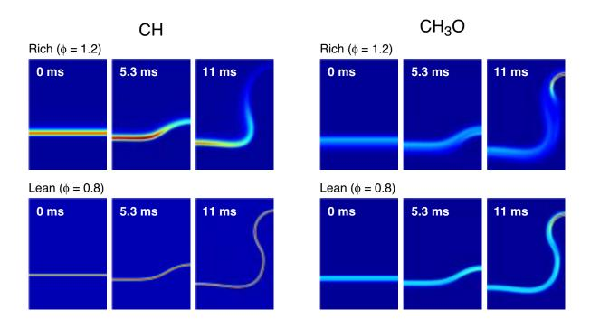
Figure 5: Behavior of CH and CH<sub>3</sub>O during vortex flame interaction for  $\phi = 0.8$  and 1.2
