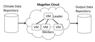
Figure 3: Design of leader election-based virtual Machine
