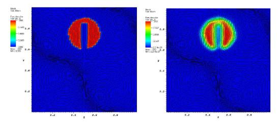
Fig. 14. Circular advection of a slotted cylinder on a  $100 \times 100$  deformed grid (84). The left is the initial condition (and reference solution), and the right is the computed solution after one revolution. The slot and bridge do fill in and slump, respectively, but the overall agreement is good.
