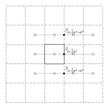
Fig. 1. Stencil for  $\langle \partial \Phi / \partial \xi_d \rangle_{\mathbf{i} + \frac{1}{2} \mathbf{e}^d}$ . The values of  $\Phi$  at the cell centers marked by the open circles determine the  $\beta$  values given by (29) at the cell faces marked by the solid circles.
