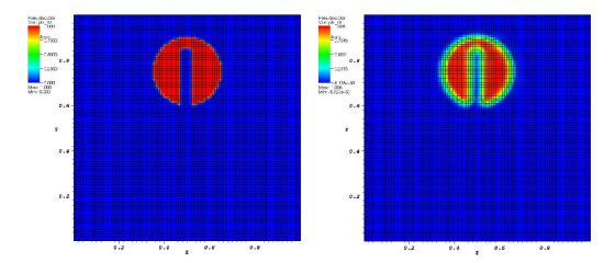
Fig. 13. Circular advection of a slotted cylinder on a  $100 \times 100$  Cartesian grid. The left is the initial condition (and reference solution), and the right is the computed solution after one revolution. The slot and bridge do fill in and slump, respectively, but the overall agreement is good.
