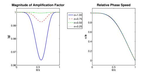
Fig. 7. Variation of the magnitude of the amplification factor |g| and the relative phase speed  $\alpha/a$  with phase angle  $\theta$  for several values of  $\sigma$ . Note that as  $\theta \to \pm \pi$ , the damping vanishes and the modes do not propagate. Furthermore, the phase error is effectively independent of  $\sigma$ .
