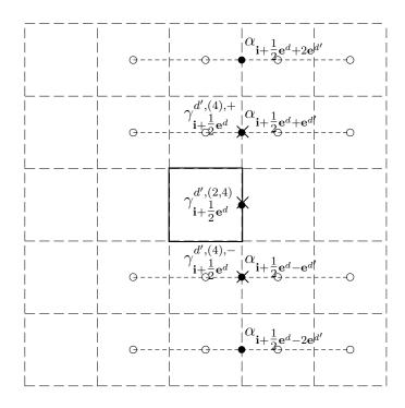
Fig. 2. Stencil for  $\langle \partial \Phi / \partial \xi_{d'} \rangle_{\mathbf{i} + \frac{1}{2} \mathbf{e}^d}$  with  $d' \neq d$ . The values of  $\Phi$  at the cell centers marked by the  $\circ$  symbols determine the  $\alpha$  values at the  $\bullet$  symbols via (34), which in turn determine the  $\gamma$  values at the  $\times$  symbols defined by (37)–(39).
